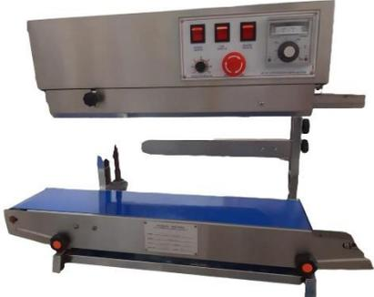
A laboratory-grade continuous sealer for Teflon tape. It features a grey top housing with three red power buttons and a control knob. The base is blue and includes a cutting mechanism and a support stand. | <p>Selladora continua de bandas de teflón</p> |
