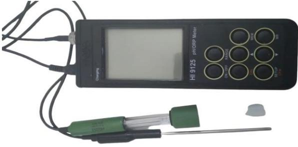
A digital pH meter with a black body and a green electrode. The device has a small LCD screen and several buttons. The text "HI 9125 pH/mV/Temp Meter" is visible on the front panel.                        | <p>pH metro marca HANNA</p>                   |
